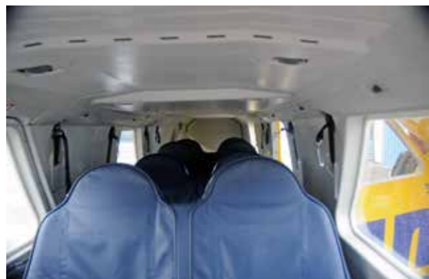
The Islander's cabin is fitted with nine passenger seats, including one alongside the single pilot.
